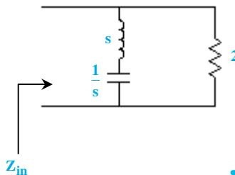
$$Z_{in}(s) = \left(s + \frac{1}{s}\right) \parallel 2 = \frac{\frac{(s^2 + 1)}{s}}{s + \frac{1}{s} + 2} = \frac{2(s^2 + 1)}{s^2 + 2s + 1}$$
