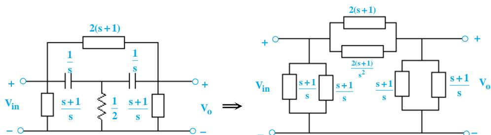
$$V_o = \frac{\left(\frac{s+1}{s}\right)\left(\frac{s+1}{s}\right)}{\left(\frac{s+1}{s}\right)\left(\frac{s+1}{s}\right) + 2\left(\frac{s+1}{s}\right) + \frac{2(s+1)}{s^2}} = \frac{\frac{s+1}{s}}{\frac{s+1}{s} + \frac{2(s+1)}{s^2} + \frac{2(s+1)}{s^2}} = \frac{s+1}{s^2 + 4s + 1}$$
