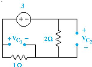
$$V_{C_1}(0^-) = \frac{1}{1+2} \times 3 = 1V$$
