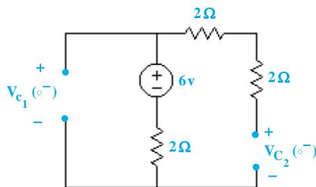
$$\Rightarrow V_{C_1}(0^-) = V_{C_2}(0^-) = 6V$$
