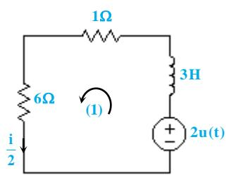
$$\text{KVL}_1 : \gamma \times \frac{i}{2} + \gamma \frac{i'}{2} = 2u(t) \Rightarrow i = ke^{-\frac{\gamma}{3}t} + \frac{4}{\gamma}$$
