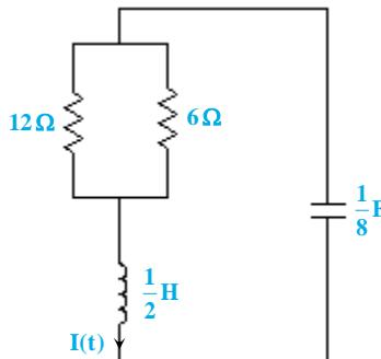
$$\text{KVL: } \frac{6 \times 12}{6+12} I + \frac{1}{2} \frac{dI}{dt} + 1 \int_0^t Idt = 0 \rightarrow \frac{d}{dt} \left( \frac{4dI}{dt} + \frac{1}{2} \frac{d^2 I}{dt^2} + 16I \right) = 0 \\ \Rightarrow \frac{d^2 I}{dt^2} + \frac{1}{2} \frac{dI}{dt} + 16I = 0$$
