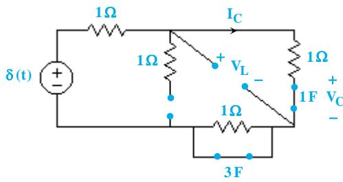
$$I_0(0^+) = I_0(0^-) + \frac{1}{L} \int_{0^-}^{0^+} V_L(t) dt = \frac{1}{2} \int_{0^-}^{0^+} V_L(t) dt$$
