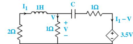
$$\xrightarrow{(1),(2)} \frac{1}{\Delta} \frac{d}{dt} \left( -V I_1 - \frac{dI_1}{dt} \right) + \frac{1}{C} (I_1 + 2I_1 + \frac{dI_1}{dt}) + \frac{dI_1}{dt} = 0$$
