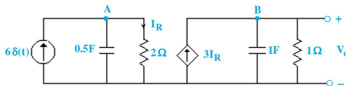
$$V_C = 2I_R \Rightarrow \text{KCL}(A) : I_R + \frac{1}{\gamma} \frac{d}{dt}(2I_R) = 6\delta(t) \Rightarrow \frac{d}{dt} I_R + I_R = 6\delta(t) \quad (1) \quad , \quad I_R(0^-) = 0$$
