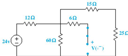
$$V_C(o^-) = \frac{60 \parallel (15+25)}{12+60 \parallel (15+25)} \times 24 \Rightarrow V_C(o^-) = \frac{24}{24+12} \times 24 = 16V \rightarrow \text{گزینه} (1) \text{ صحیح است}$$
