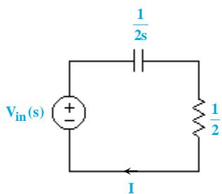
$$I(s) = \frac{V_{in}(s)}{\frac{1}{2s} + \frac{1}{2}} = \frac{2s V_{in}(s)}{s+1}$$
