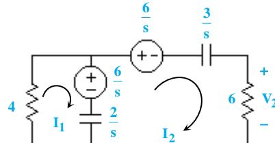
$$\text{KVL(1)}: \frac{6}{s}I_1 + \frac{6}{s} + \frac{6}{s}(I_1 - I_2) = 0 \Rightarrow (6s + 2)I_1 - 6I_2 = -6 \quad (1)$$
