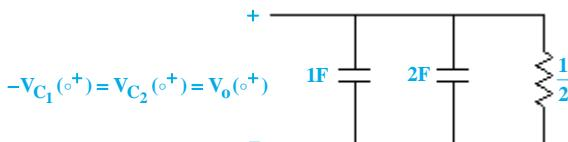
$$V_o(0^+) = \frac{c_2 V_{C_2}(0^-) - c_1 V_{C_1}(0^-)}{c_1 + c_2} = \frac{2 \times 5 - 1 \times 5}{2 + 1} = \frac{5}{3}V$$
