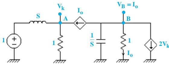
$$\text{KCL}(A): \frac{V_k - 1}{s} + V_k = I_o \Rightarrow (s+1)V_k - sI_o = 1 \quad (1)$$
