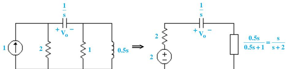
$$V_o = \frac{\frac{1}{s}}{\frac{1}{s} + \frac{1}{2} + \frac{1}{s+2}} \times 2 = \frac{2s + 4}{3s^2 + 5s + 2} \xrightarrow{s=j\omega} V_o(j\omega) = \frac{4 + 2\omega j}{2 - 3\omega^2 + 5\omega j}$$
