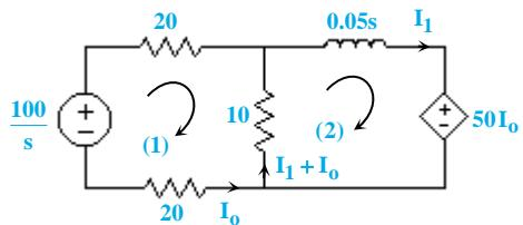
$$\left\{ \begin{array}{l} kvl(1): 50I_0 + 10I_1 = -\frac{100}{s} \\ kvl(2): (\frac{10}{20} \Delta s + 10)I_1 + 10I_0 = -50I_0 \end{array} \right. \quad (1)$$
