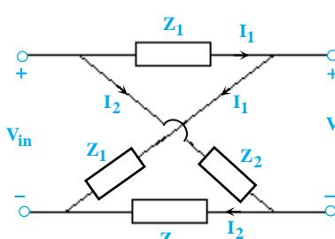
$$V_{in} = 2Z_1 I_1 = Z_2 I_2 + Z_1 I_1 \Rightarrow I_2 = \frac{2Z_1}{Z_1 + Z_2} I_1 \quad (۱)$$
