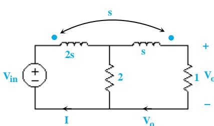
$$kvl(\text{حلقه چپ}): -V_{in} + (2s + 2)I - (s + 2)V_o = 0 \Rightarrow (2s + 2)I - (s + 2)V_o = V_{in}$$
