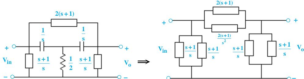
$$V_o = \frac{\left(\frac{s+1}{s}\right) \parallel \left(\frac{s+1}{s}\right)}{\left(\frac{s+1}{s}\right) \parallel \left(\frac{s+1}{s}\right) + 2(s+1) \parallel \frac{2(s+1)}{s^2}} = \frac{\frac{s+1}{s}}{\frac{s+1}{s} + \frac{2(s+1)}{s^2}} = \frac{s+1}{s^2 + 4s + 1}$$
