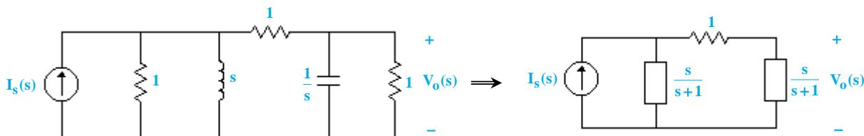
$$\Rightarrow V_o(s) = \frac{\frac{1}{s+1}}{\frac{1}{s+1} + \frac{1}{s+1} + \frac{1}{s+1}} \times \frac{s}{s+1} I_s(s) = \frac{1}{2} \times \frac{s}{s+1} I_s(s)$$
