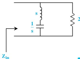
$$Z_{in}(s) = \left(s + \frac{1}{s}\right) \parallel 2 = \frac{\frac{s^2 + 1}{s}}{s + \frac{1}{s} + 2} = \frac{s^2 + 1}{s^2 + 2s + 1}$$
